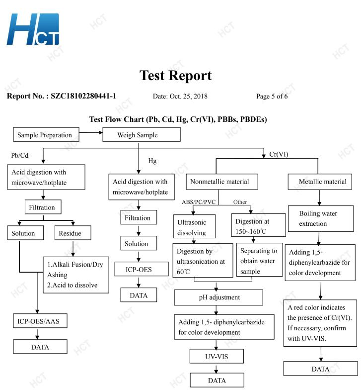
These sample were dissolved totally by pre-conditioning method according to above flow chart(Cr(VI) test method excluded)
